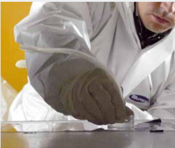
phase 2 particle sample taken of the deposit of dust inside the duct according to the NADCA Vacuum Test
