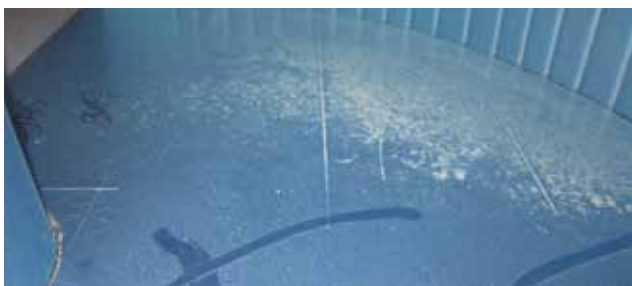
Detail of the dust deposited inside a care P3ductal duct stored in a job site
