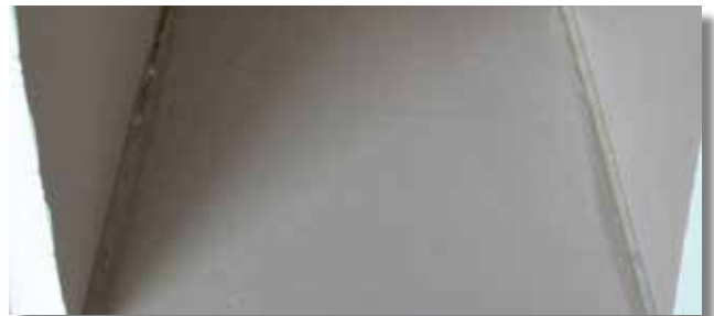
Detail of the dust deposited inside a careplus P3ductal duct stored in a job site
