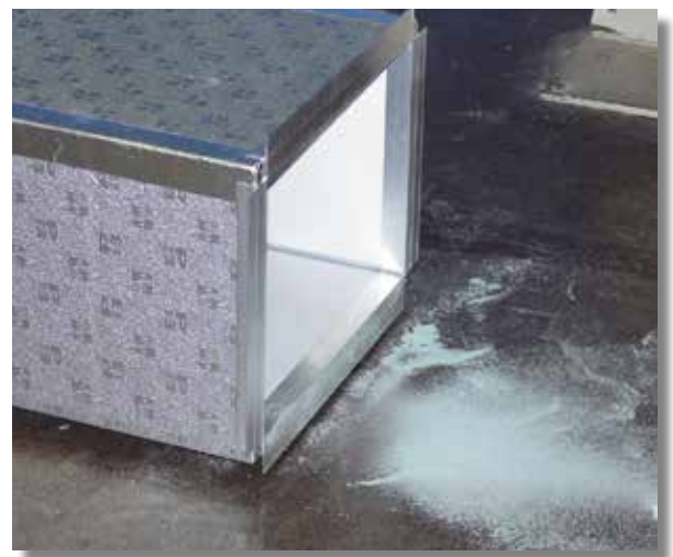
large scale test, insertion of the dust particles in the system
