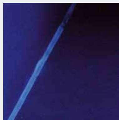
detail of the residual dirt highlighted by the Wood lamp in the proximity of the corner of the P3ductal careplus duct
