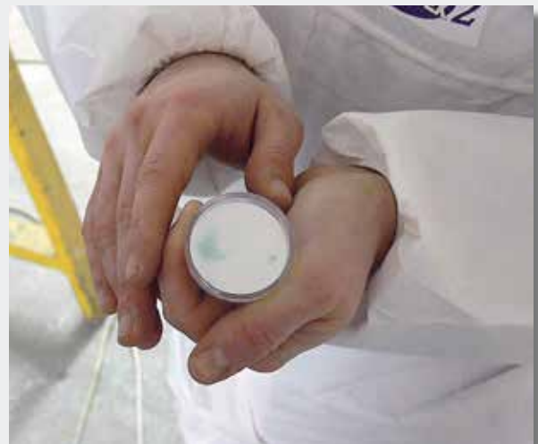
phase 3 detail of the residual dirt taken from inside the sample of sheet metal duct
